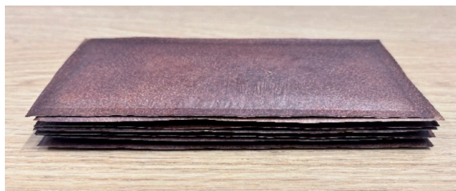
Fig. 10. Five perforated pads with external dimensions of approx. 170 × 75 mm, composed of a CTMP core (thickness approx. 1–2 mm) and covered by two METNIN™ SHIELD-treated films based on Enz-TMP 2000.
