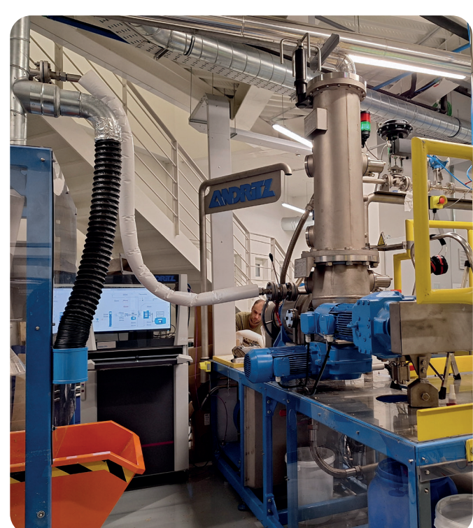
TMP Production in high-pressure Refiner
