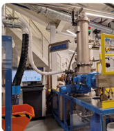
TMP Production in high-pressure Refiner
